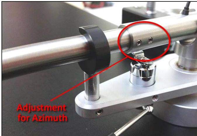
*You may adjust azimuth by loosening the side screws and turning the armtube.*
