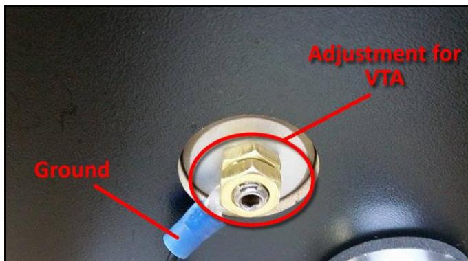
*Loosen the nut under the tone arm-base, remove the ground wire, then you may adjust the height by turning the brass nut.*
